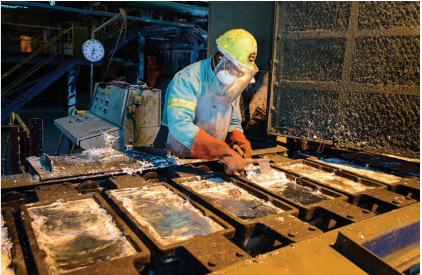
Skimming of final metal ingot production
