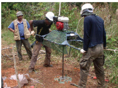
To better define drill targets, power augers are used to sample saprolite soils up to 10 meters deep.
