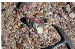
Visible Copper Mineralisation (malachite) near the Canbelego Copper Mine, NSW
