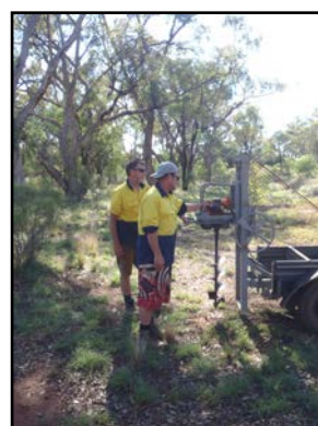
Quad bike towed Auger Team sampling, NSW
