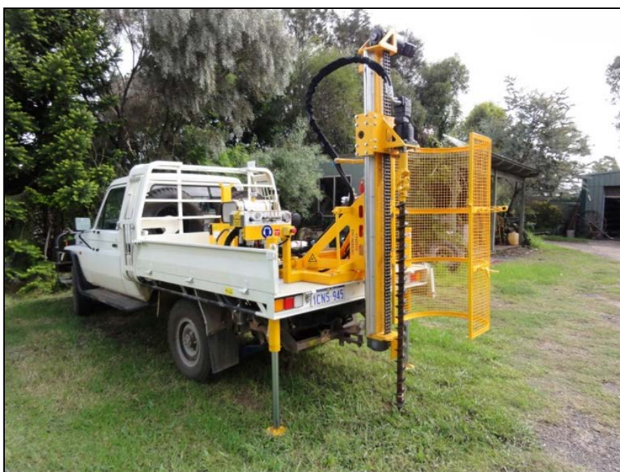
Figure 7: Helix Auger Rig will allow our field team to sample a consistent soil horizon across areas of variable cover (up to max 20m). This will be used to identify drill targets on the southern extensions of the Tritton and Kurrajong VMS trends to work up targets for drill testing.
