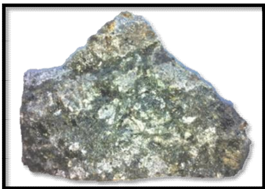
Figure 2a) Brecciated Dacitic Porphyry with disseminated chalcopyrite and chalcocite from the base of the Carmelita workings (~50m below surface) on the eastern edge of Target 1. Sample assayed 3.1% Cu, 0.1g/t Au, 11g/t Ag and 200ppm Mo 1 .
