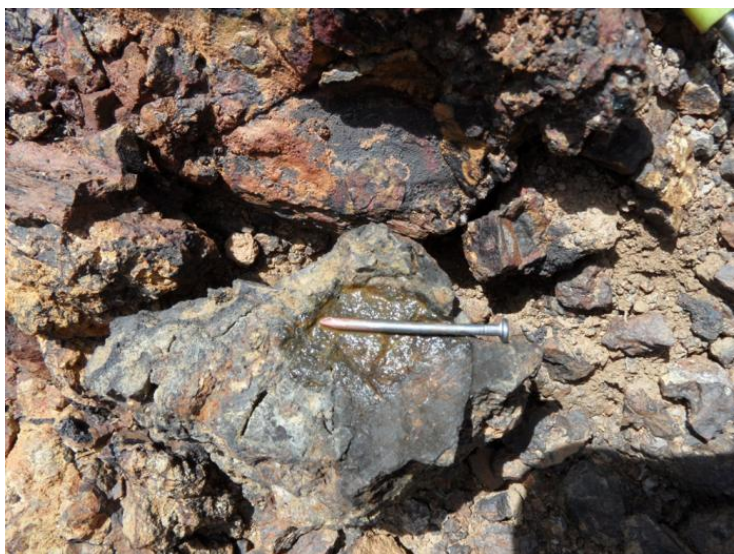
Figure 6: Extensive stockwork present at the Samuel Prospect containing limonite after sulphides. Rock sample 55795 returned 0.03 ppm Au, 4125 ppm Cu, 36 ppm Mo
