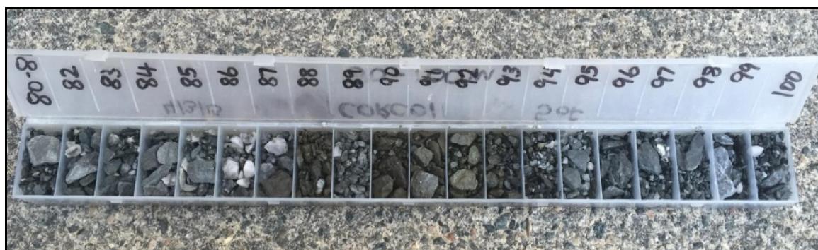
Figure 10: CORC011 – 10m @ 2.6% Cu from 84m incl. 7m @ 3.2% Cu, 1.7% Zn, 11g/t Ag from 86m (Refer ASX Announcement on 1 April 2015) 2
