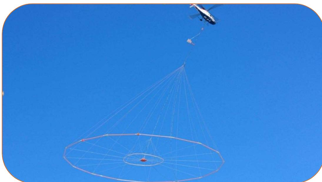
**Figure 7: VTEM MAX<sup>TM</sup> system in flight (Photo – Geotech)**
