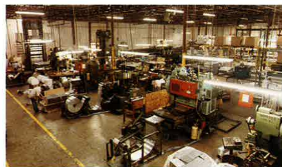
Fin press and tube expanding area.
