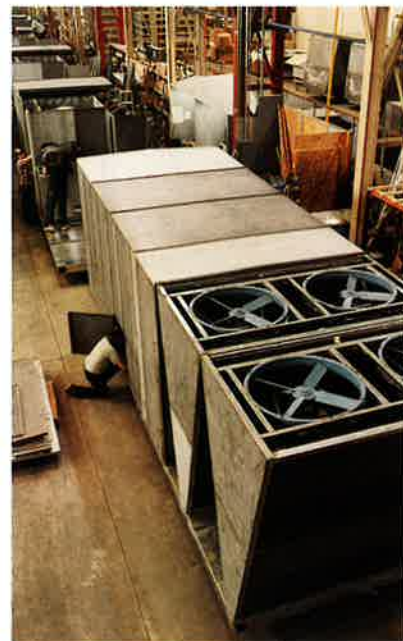
Production line No. 3 showing a series of 8, 140 ton units.
