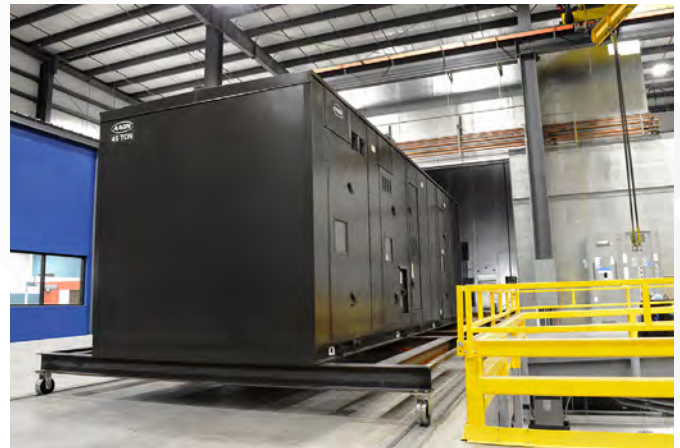
45 ton AAON Water-Source Heat Pump Rooftop Unit being moved into the 50 ton Psychrometric Chamber
