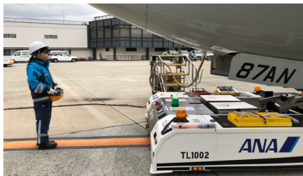
Pushback using Mototok EVs
