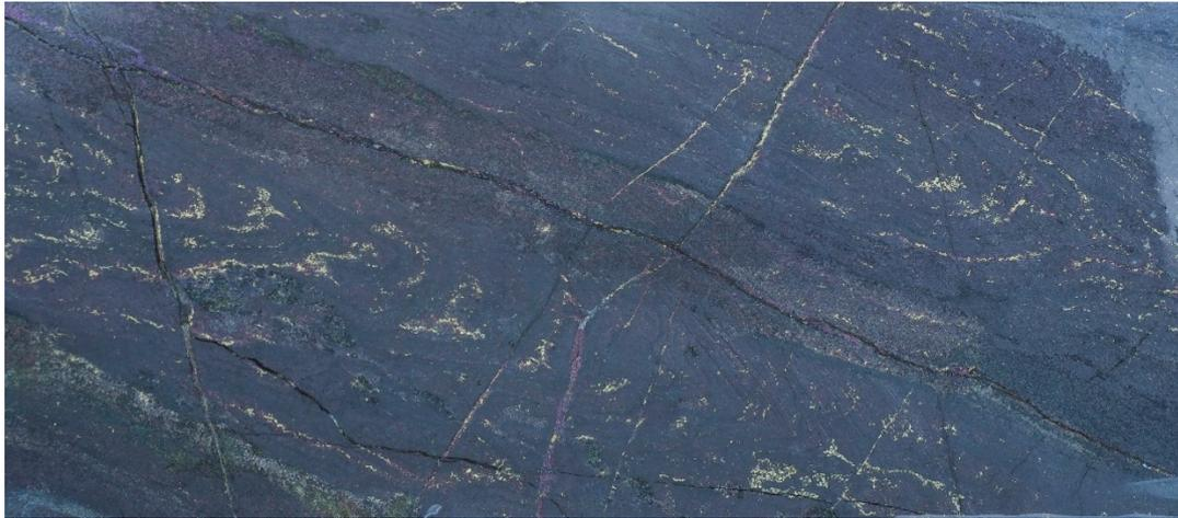
Figure 6: Chalcopyrite replacing folded, crenulated bedding planes in magnetite rich skarn, hole ZX-18023
