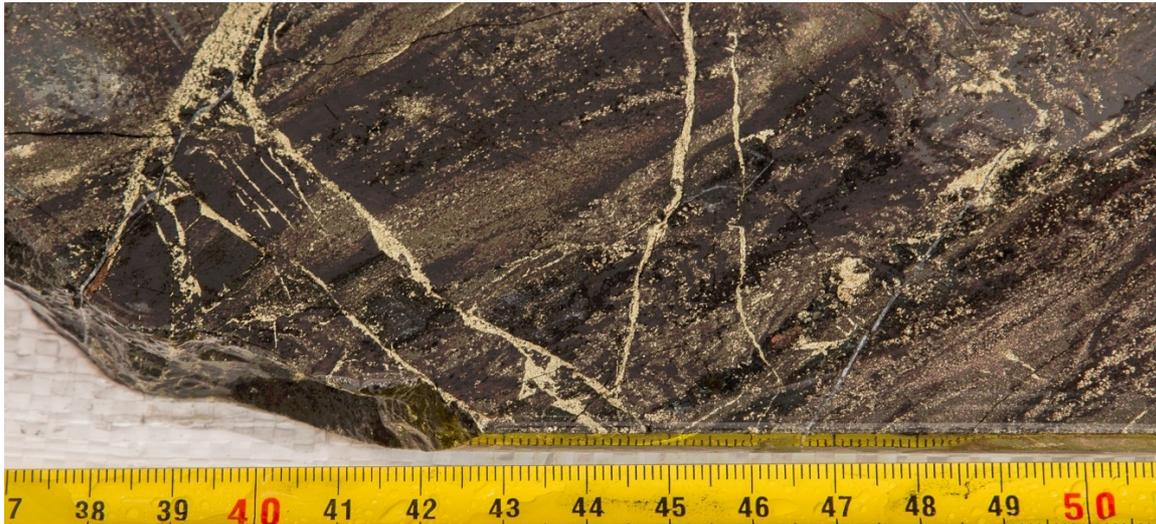
**Figure 8:** Visible copper sulphides and magnetite in half-core, hole ZX-18025, 93.9m down-hole depth. Copper sulphides comprise mainly chalcopyrite (yellow colour). Assays returned mineralisation grades of 5.4% Cu, 3.7g/t Au and 16.3g/t Ag for the interval including the above core-photograph. Scale bar is in cm
