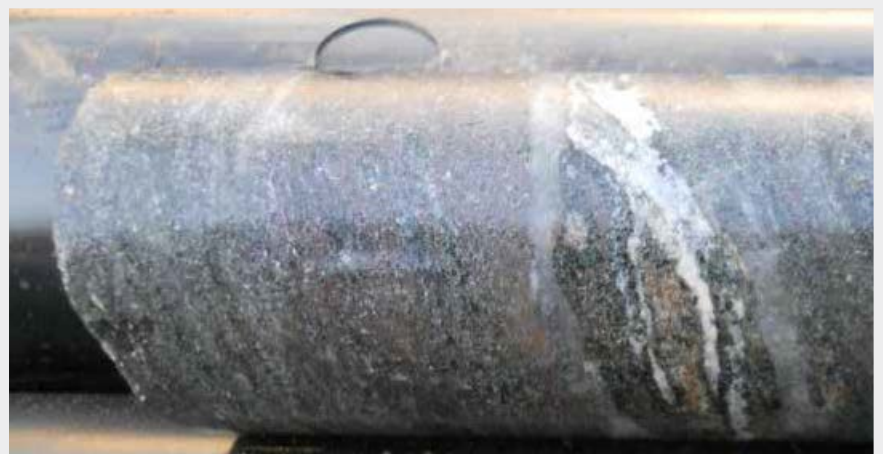
Figure 11: 5cm band of sphalerite with minor galena in PAD001 80-81
