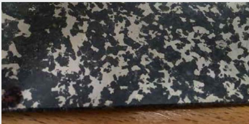
◀ Figure 5: Polished NQ Core from 45.5m AKD009 showing pyrrhotite mineralisation and minor pentlandite
