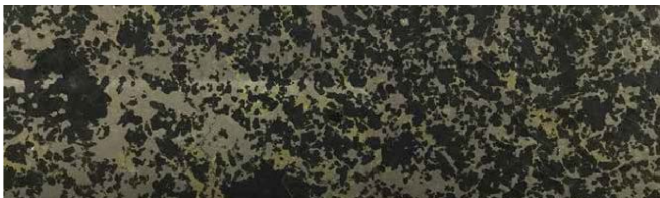
Figure 9: Close-up of matrix textured sulphides in NQ core 218m AKD017 showing chalcopyrite (Cu), pyrrhotite (Fe) and pentlandite (Ni)
