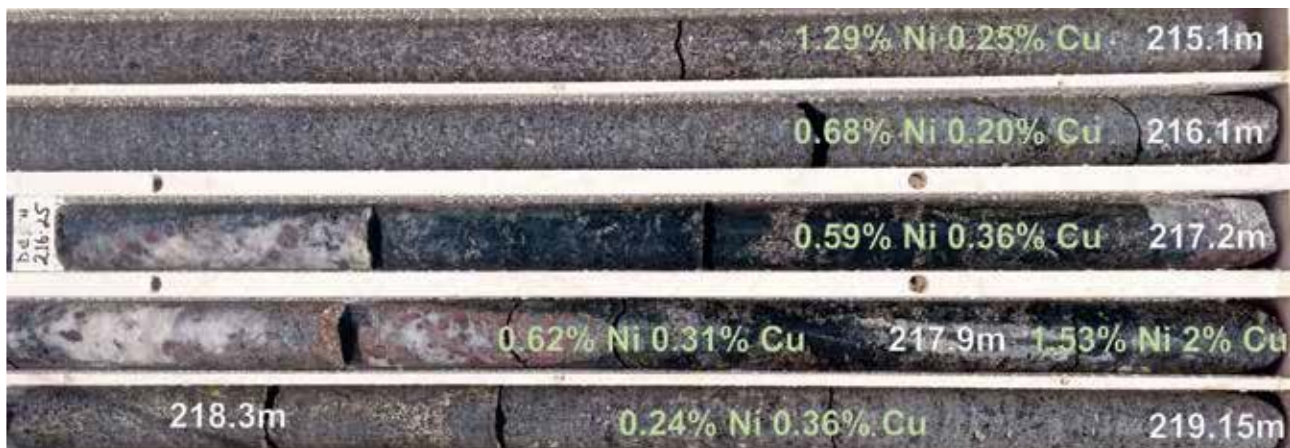
Figure 8: Mineralised NQ core from AKD017 part of 5.2m interval from 213.1m to 218.3m showing matrix textured sulphides averaging 1% Ni and 0.41% Cu
