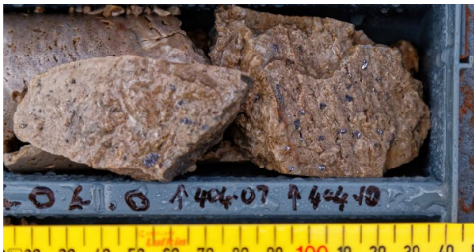
Disseminated galena in dolomitised Pillara Limestone at 404.07m in hole BWTDD0003, with up to 1.34% lead recorded in spot pXRF readings. Core diameter is 47mm.
