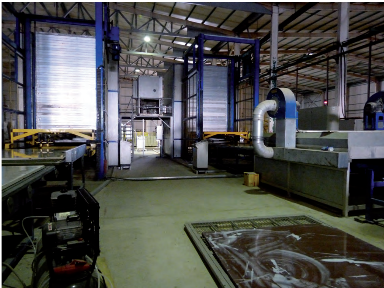
Figure 9 – View of the resin ovens in the factory allowing slabs to be treated prior to polishing. In the foreground a slab of Rosso Cait with resin freshly applied waits to be added to the line.
