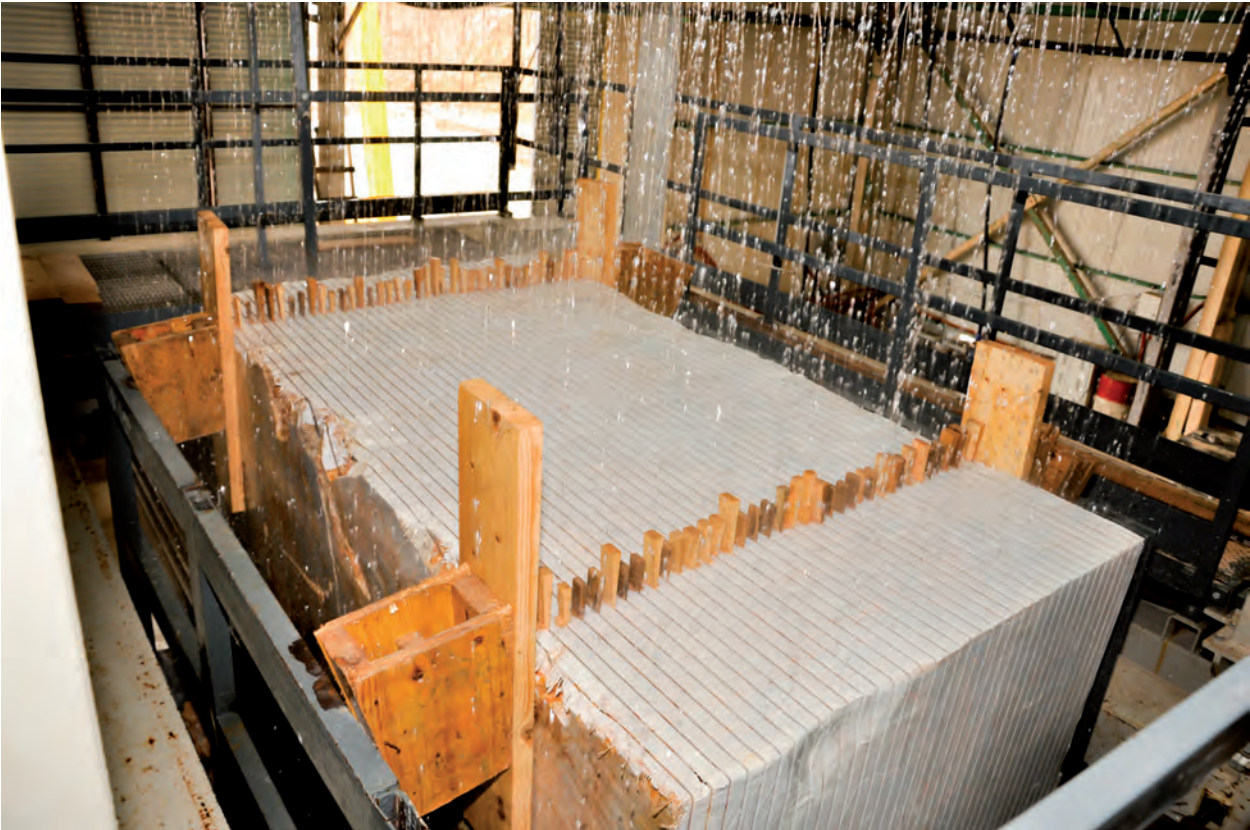
Figure 3 – Breccia Paradisea block nearing the end of its cut on a gang saw in Fox Marble factory
