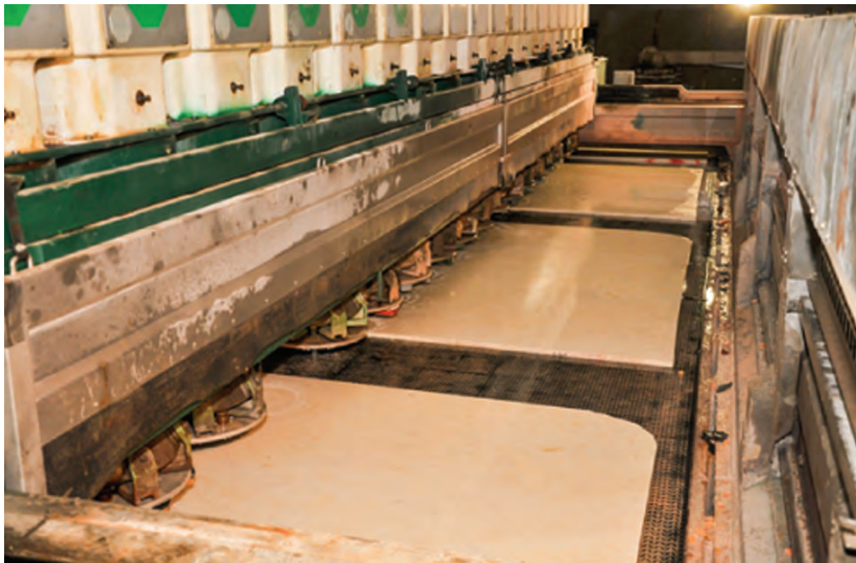
Figure 10 – Three slabs of Illirico Bianco being polished in the Fox Marble factory. Polishing heads rotate at high speed across the slabs to provide high quality finish.
