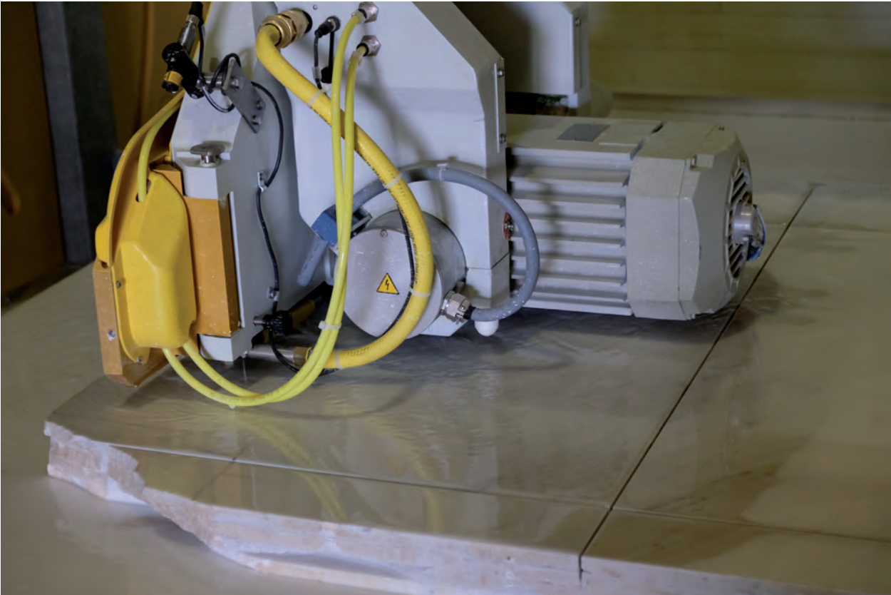
Figure 5 – CNC machine cutting marble tiles to size
