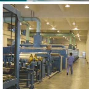
Stentering line reduces fabric shrinkage, China
