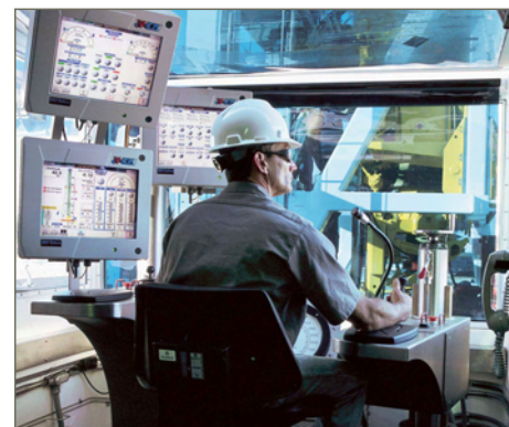
The driller controls the FlexRig's operation from a controlled climate cabin using touch screens and joystick controls.
