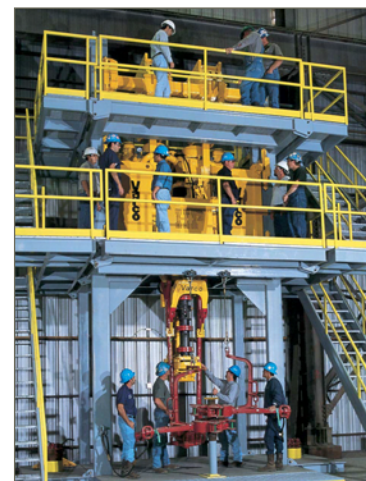
Our instructors and crews use a unique training aid to develop top drive skills.
