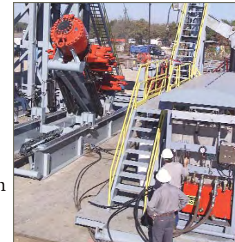
The new hydraulic blowout preventer handling system shortens a well's critical path and improves personnel safety.
