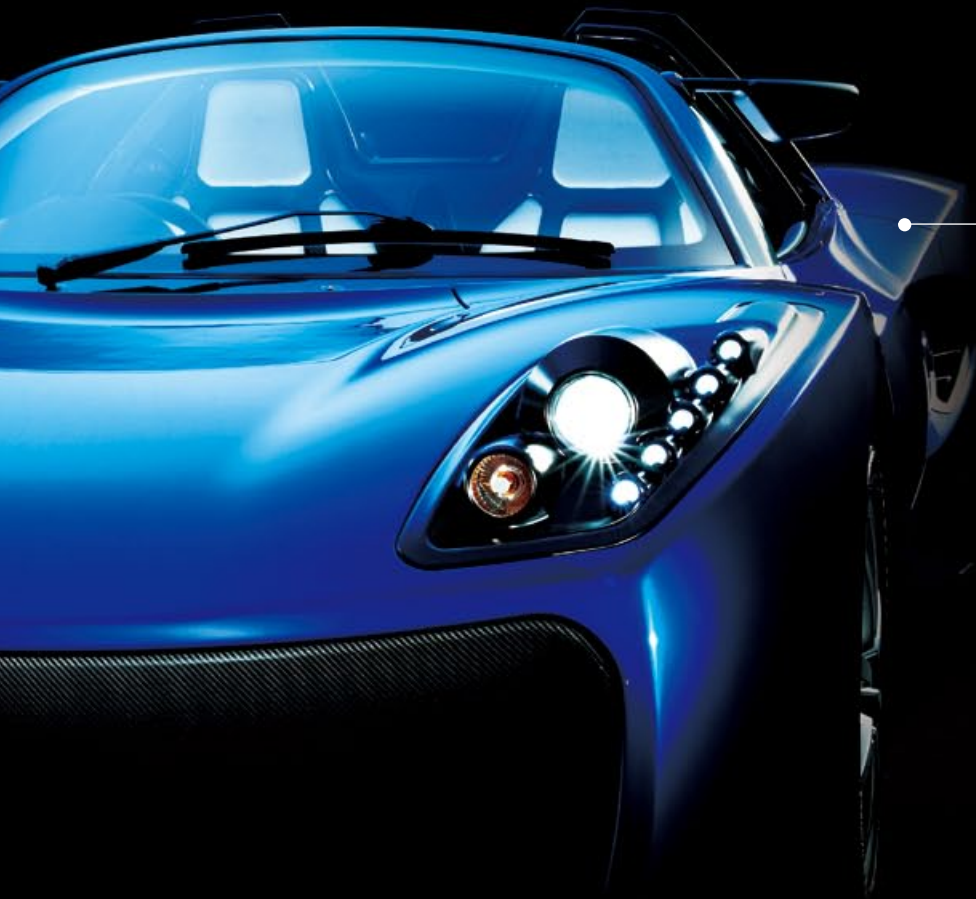
The TEEWAVE® AR1 electric vehicle concept car Toray made with a carbon fiber body in 2011
