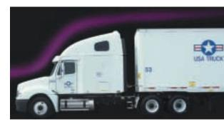
is by creating efficiencies in overall fuel consumption. Options that improve fuel economy are specified in our new Columbia class tractor orders. The aerodynamic body design of the new Columbia and new advances governing miles per hour contributes to optimum fuel efficiencies on the open road. In addition, the Columbia class features "Optimized Idle" settings which further increase fuel efficiencies. Each tractor
