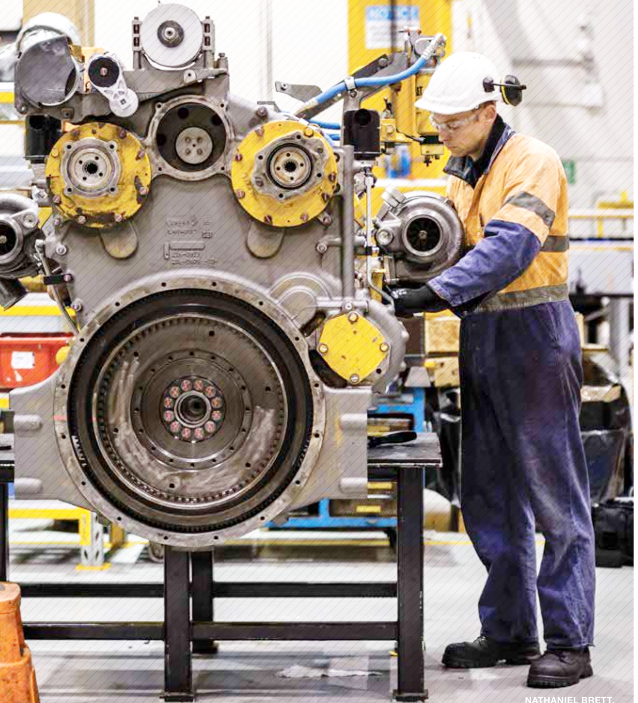
NATHANIEL BRETT, TEAM LEADER CRC ENGINE SECTION IN TOMAGO, TENSIONING THE TURBOCHARGER MOUNTING BOLTS ON A CAT C32 ENGINE.
