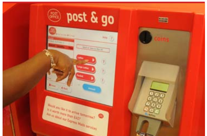
Automated Post & Go machines enable customers to weigh and pay for postage away from the counter.
