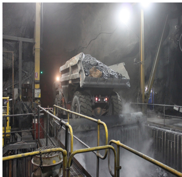
Truck Tipping at Underground Crusher
