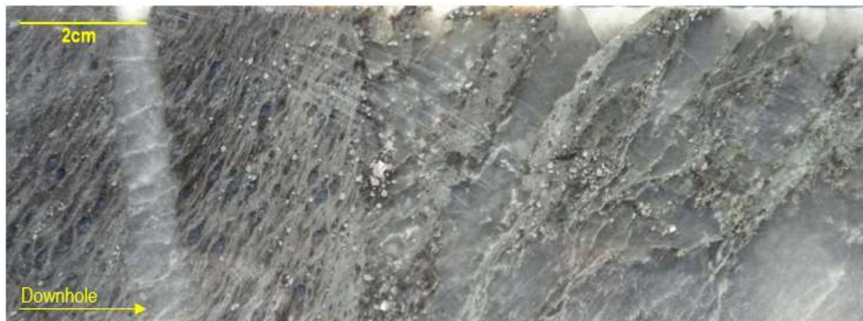
Figure 7 | Example of mineralisation in hole ARDD278 at 162.7m drill depth, returning 5.26g/t gold in highly strained quartz feldspar porphyry with sericite-pyrrhotite-arsenopyrite alteration in selvage of quartz-chlorite-arsenopyrite-gold veins.
