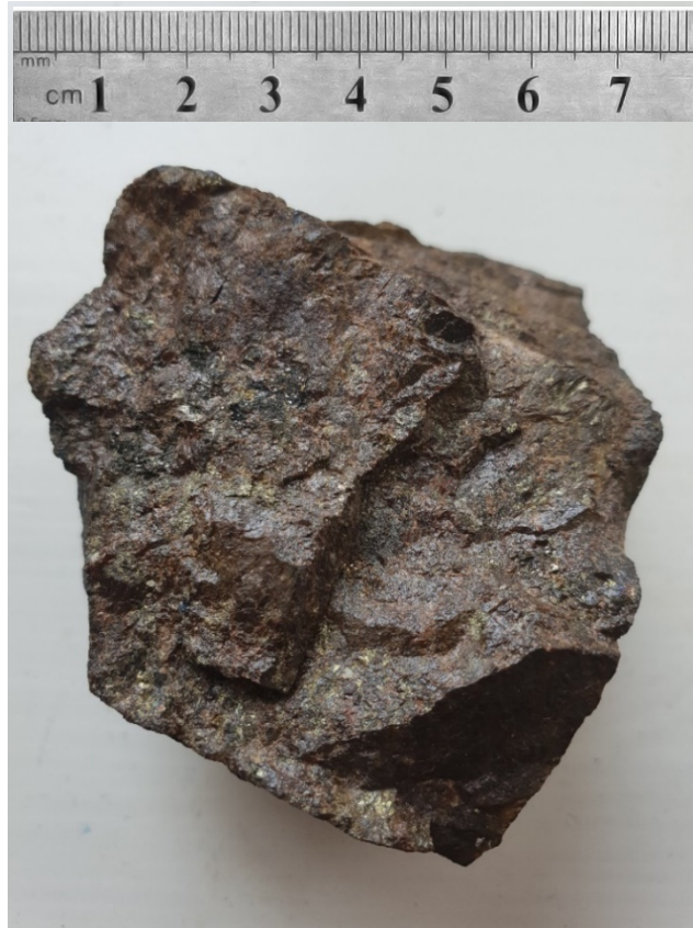
Figure 10: Stone Lake chalcopyrite-pyrrhotite-pyrite mineralisation in massive garnet skarn.
