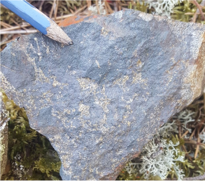
Figure 11: Heritage Valley chalcopyrite-pyrrhotite mineralisation in semi-massive magnetite and proximal skarn.
