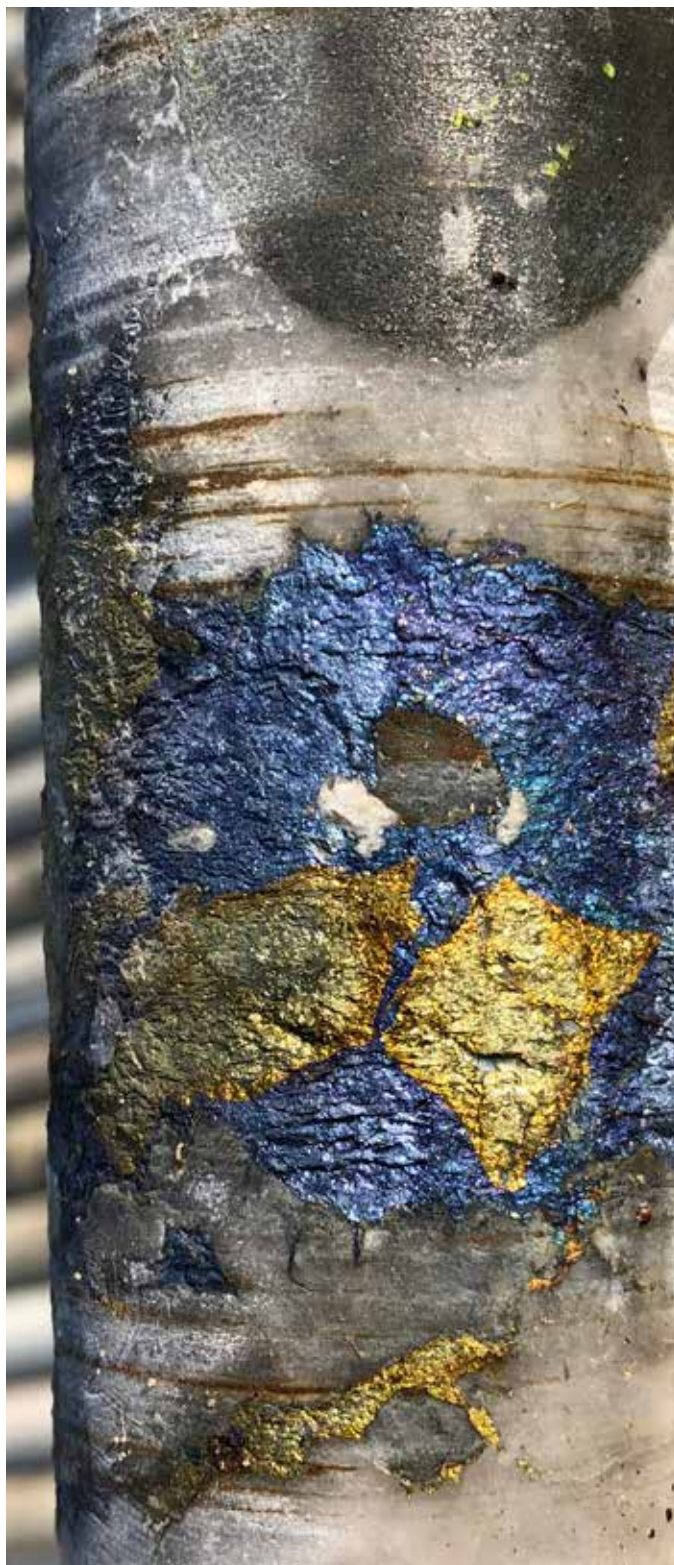
Drill core showing coarse grained bornite and chalcopyrite
