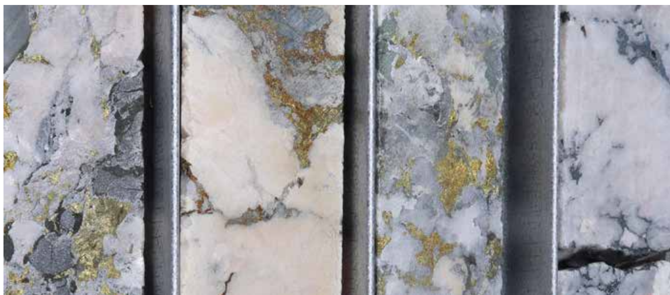
Vein hosted Cu mineralisation – mainly chalcopyrite (T23, A4, T3 & A1)
