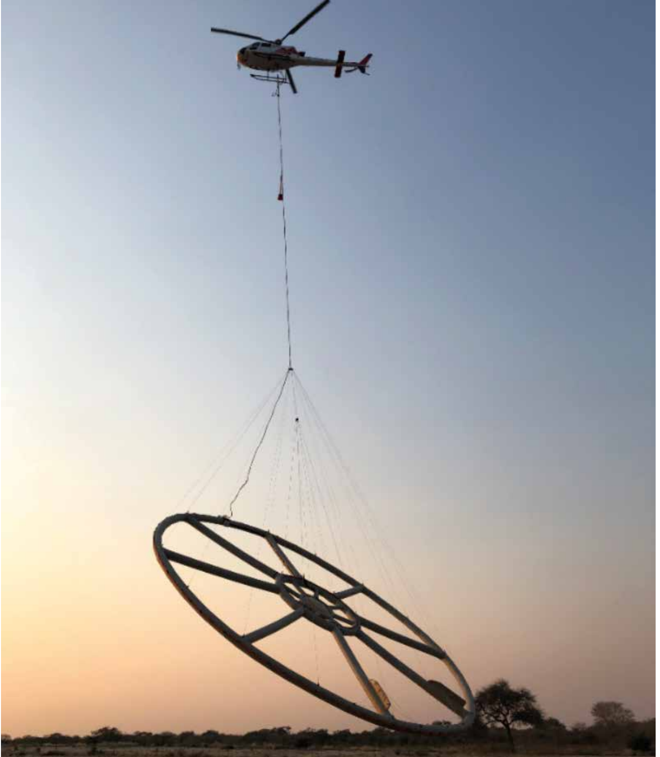
Airborne electromagnetic survey dawn take-off from field base in the Okvanago Copper Project
