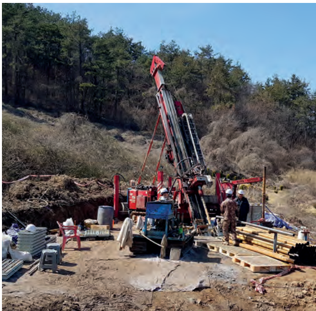
Southern Gold - Diamond drilling of BPDDH12 in progress at the Hand of Faith prospect, part of the Beopseongpo project area, targeting medium to low sulphidation epithermal vein systems with evidence of boiling textures and gold mineralisation in the target "hanging wall vein".
