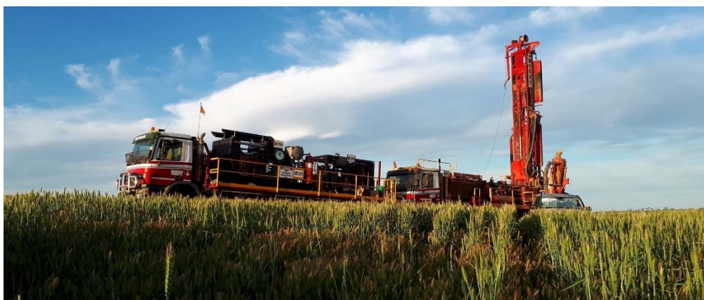
Figure 3 – RC percussion drilling at the Quicksilver Ni-Co-Cu Project
