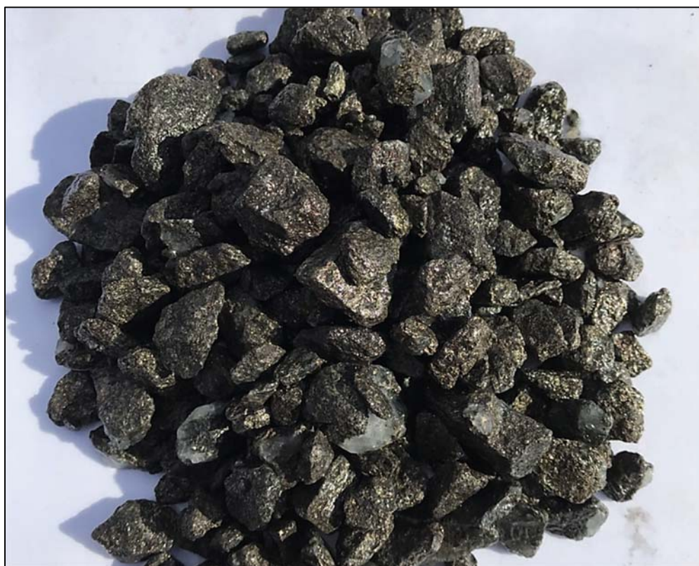
Figure 5 – Semi to Massive Sulphide from 200-202 metres downhole in QRC149
