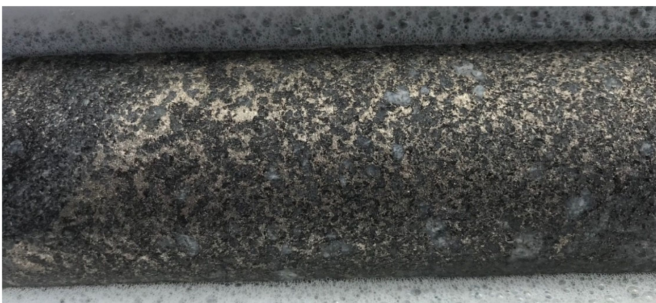
Figure 20 – Massive sulphide mineralisation from hole QDD0004, length 15cm, approximately 214 metres depth downhole
