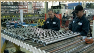
Newly installed perforating gun manufacturing cell at the Hunting facility in Calgary, Canada.
