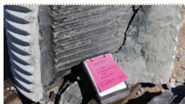
API test on a concrete core to show pattern and penetration of a perforating operation.
