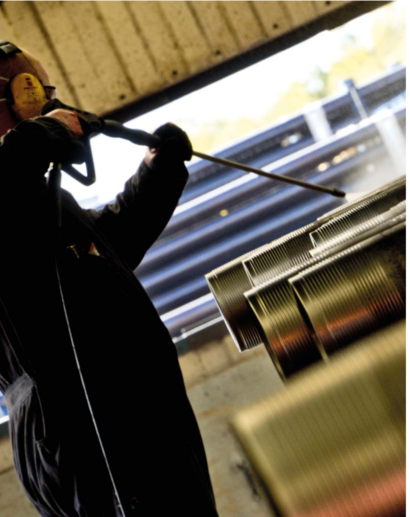
TUBING BEING PREPARED FOR INSPECTION, REPAIR AND RETURN TO SERVICE IN THE NORTH SEA.
