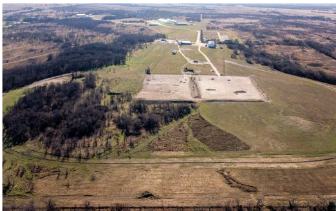
THE FLOW LOOP AT TITAN'S MILFORD TEST FACILITY IS A MILE LONG CONSISTING OF 5½ INCH CASING.
