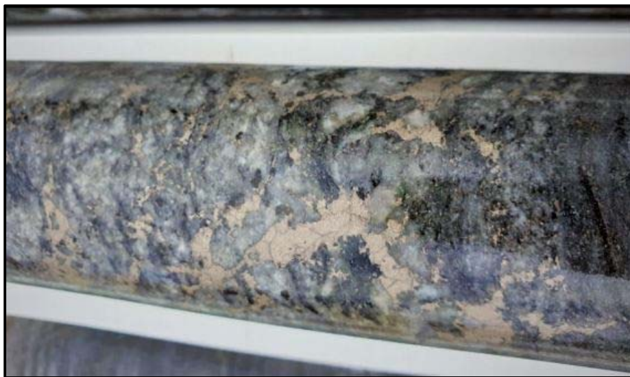
Figure 8: Sulphide stringers and veins with quartz in ER001 at 407m (field of view approximately 15cm across)
