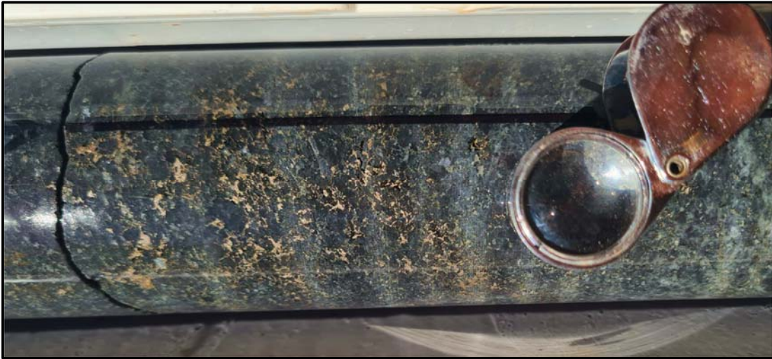
Figure 4 — Disseminated Sulphide in LADD003 at 170m (pyrrhotite with minor pentlandite/chalcopyrite)
