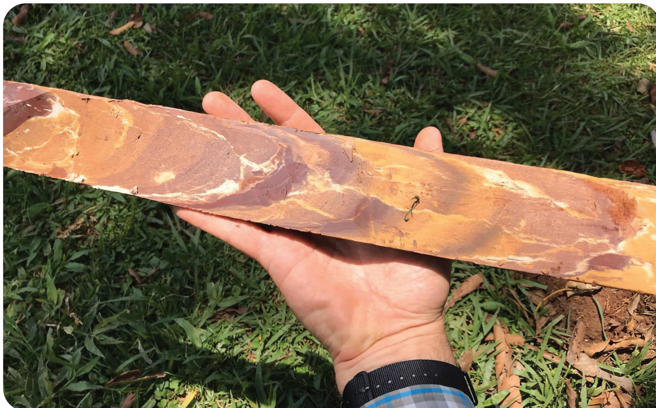
Core sample of Makuutu ionic adsorption mottled clay from hole RRMD011
