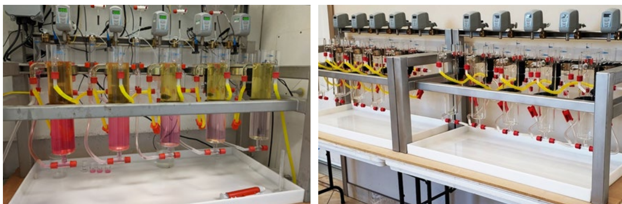
Figure 10: Mixer Settler pilot plant located at Queens University Ionic Liquids Laboratory (QUILL) at QUB.
