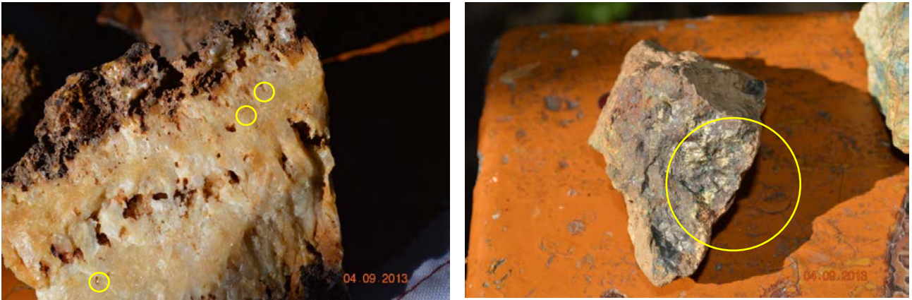
Figure 4 Rock samples containing visible gold (left) and visible chalcopyrite (right) collected from mineralised zones in the first trench. Photograph scale is approximate scale is 12cm.
