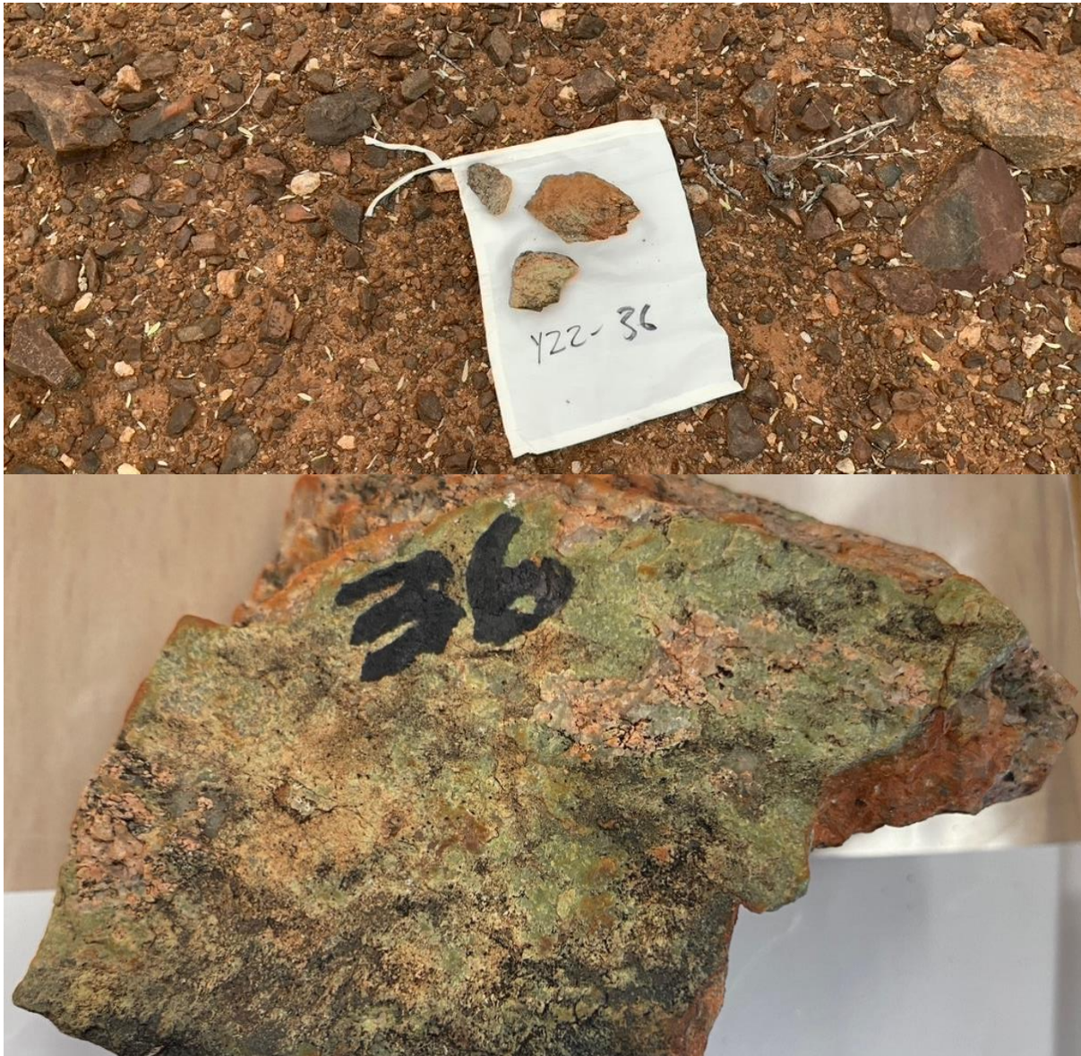
Picture 3: Yinnetharra (WCN 100%) REE/Li project, sample YZZ36 which is highly anomalous in REE's with a grade of 615ppm TREO, and thought to be proximal or near a stronger mineralised source. YZZ36 is proximal to a thorium anomaly.
