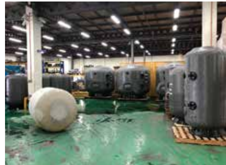
The Malaysian facility manufactures an extensive range of fibreglass filters, from 400mm to 3000mm diameter vertical filters and 860mm diameter to 2200mm diameter horizontal filters.
