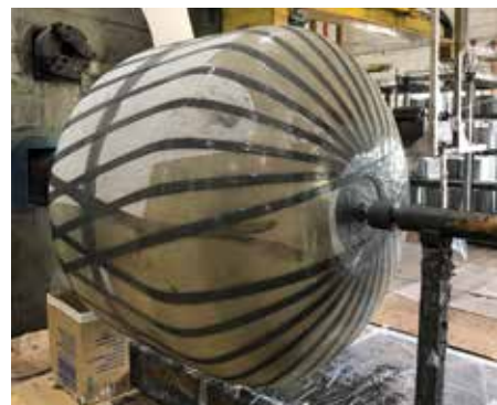
Waterco's Micron commercial fibreglass filters are made from continuous strands of high-quality fiberglass filament wound under controlled tension to create a seamless, impervious vessel.
