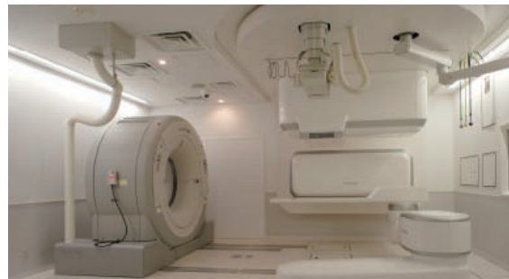
Next generation irradiation system (right) and large-bore CT (left) in the new treatment room for heavy-ion cancer therapy at the National Institute of Radiological Sciences
