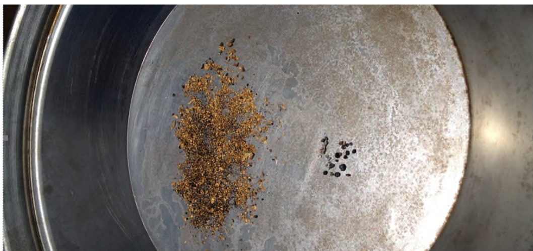
Figure 2: Gold and platinum recovered from trenching EL1968 (Sample on pan weighs approximately 10g Au and 2g Pt)
