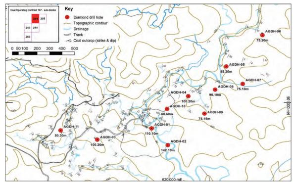
Figure 10: Coal Project - COC 197 - drill hole locations (AGDH01-AGDH11).
