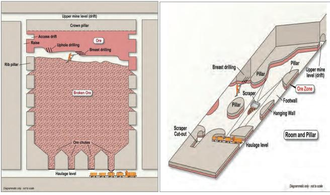
Diagram 3: Schematic diagram of a shrink stope
