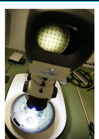
Testing and monitoring integrated circuits first at a wafer level, ensures Dialog can reach optimum production yields of a final packaged integrated circuit.
