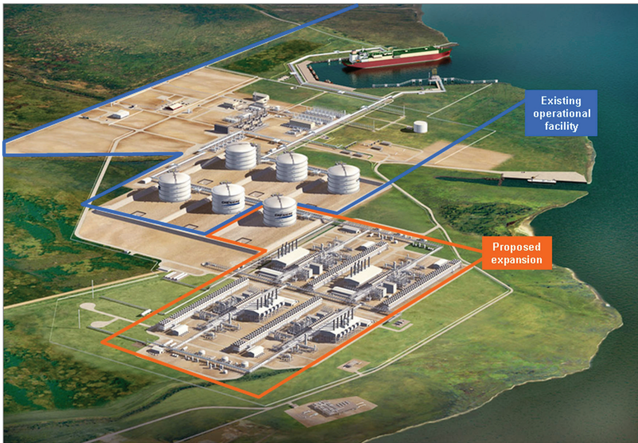
Proposed liquefaction project will transform Sabine Pass LNG into bi-directional import/export facility
