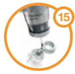
16 NC4 laser non-contact tool setting system
