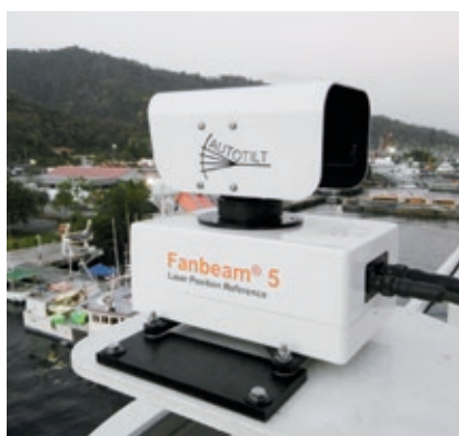
Fanbeam® 5 – the laser-based marine dynamic positioning for offshore support vessels.
