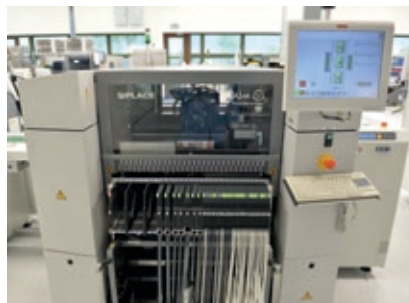
➤ The PCB assembly facility at Miskin includes technology capable of placing 40,000 components per hour.
