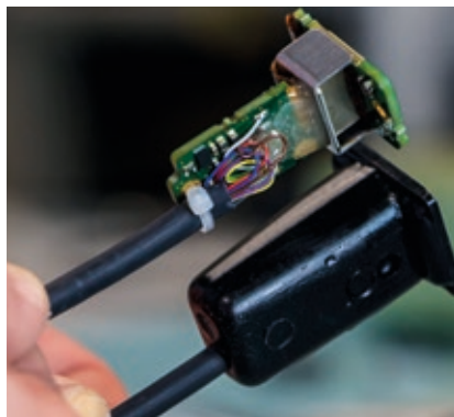
④ LinACE™ encoder from RLS repackaged into a waterproof enclosure.
