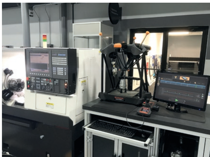
➤ The Equator™ gauge is now offered with IPC software, providing the functionality to fully automate tool offset updates in CNC manufacturing processes.
