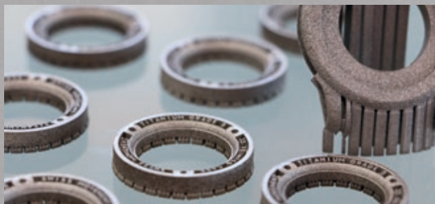
● Titanium watch cases manufactured for Holthirichs Watches using Renishaw additive manufacturing systems.
