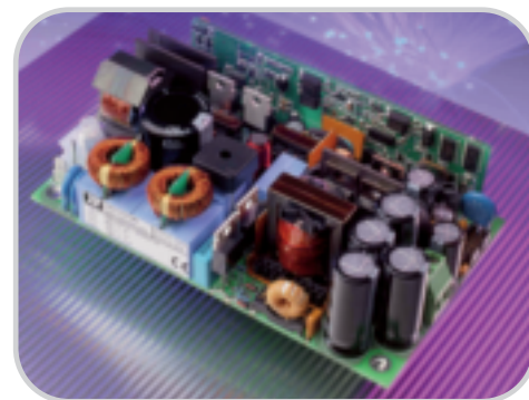
The EMA212 launched during 2006, the world's smallest commercially available 212watt power supply.
