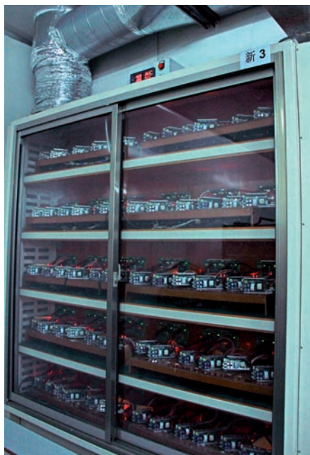
By utilising electronic loads we are able to recycle 50% of the power consumed during burn-in
