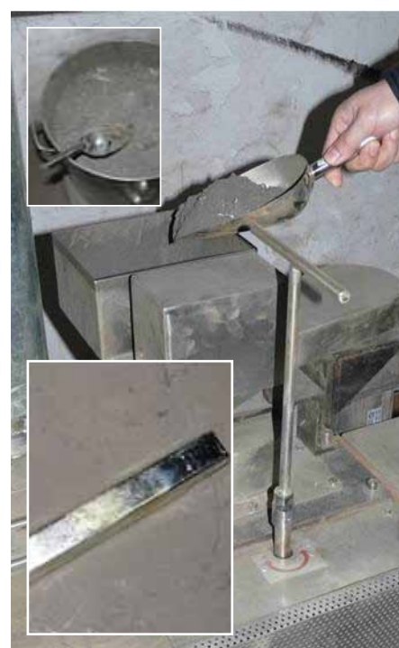
On site recycling of solder waste reduces our impact on the environment and lowers our costs. From top, Solder dross discarded from the wave soldering process, solder recycling machine and, finally, a recovered solder bar.
