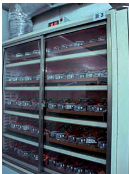
Electronic loads allow 50% of the power used during burn-in testing of the product to be recycled.
