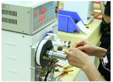
Further vertical integration by the manufacture of magnetic windings
