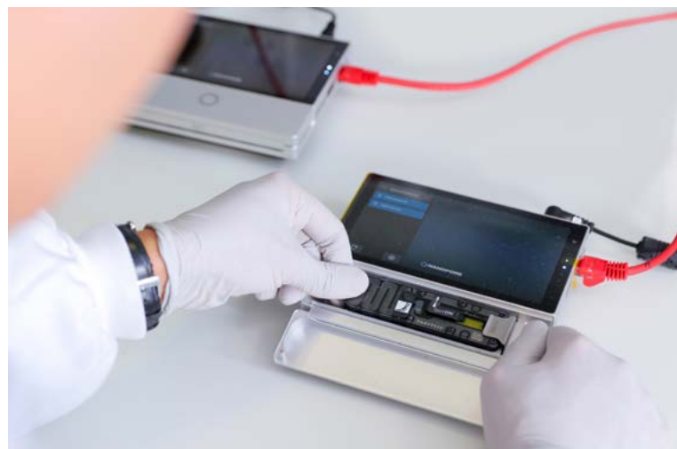
Oxford Nanopore: Scientist inserting a flow cell into MinION Mk1C
