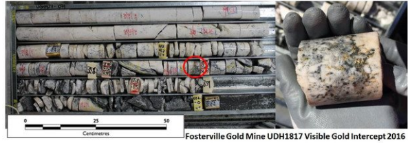
FIGURE 7-7 DRILL CORE FROM HOLE UDH1817 SHOWING VISIBLE GOLD IN A QUARTZ-CARBONATE VEIN
