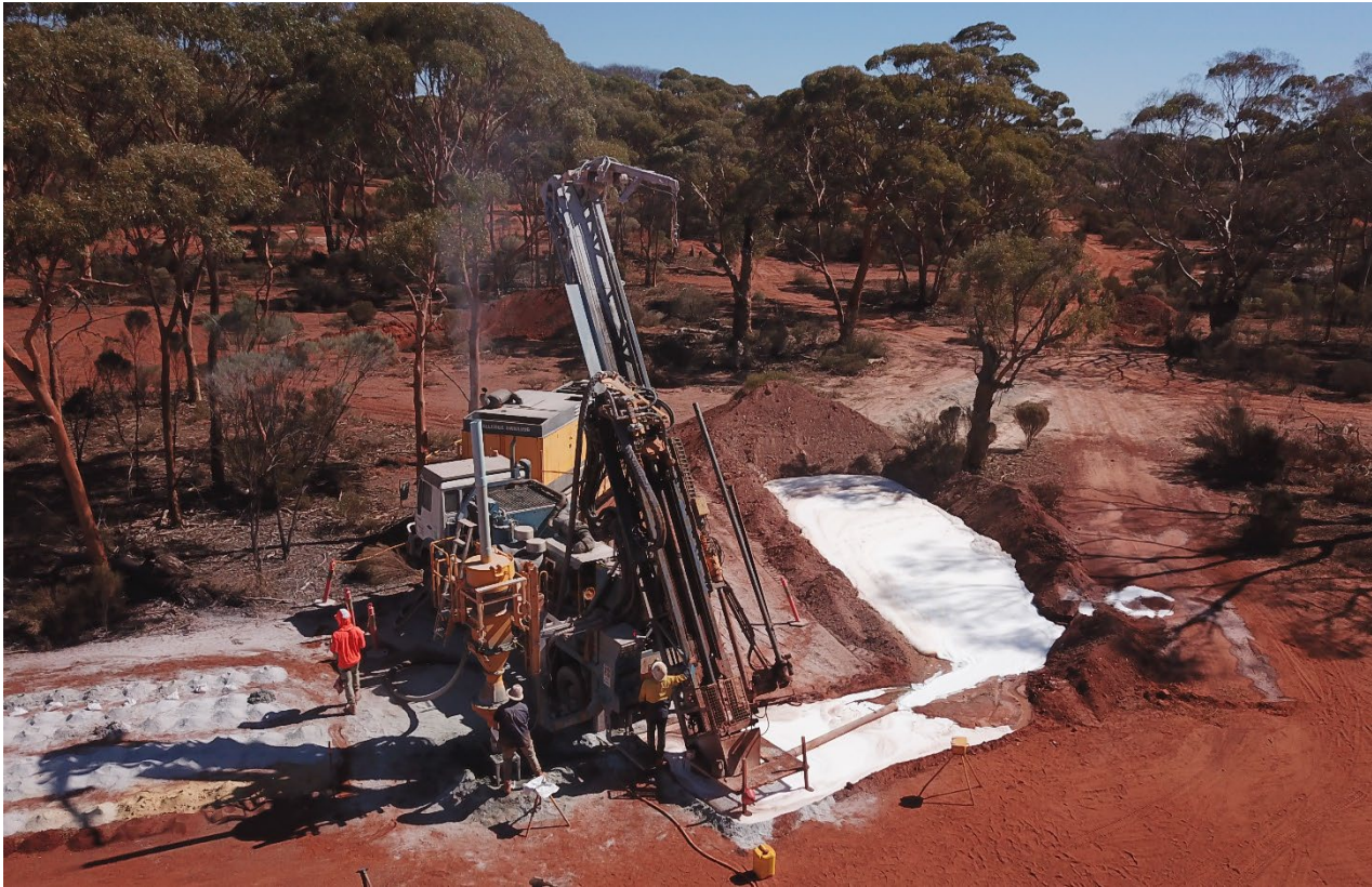
Image 1 – RC drilling at Mandilla East
